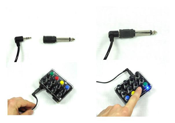
Please note that Synthino only powers on when the ¼ inch MONO plug is inserted. This acts to save battery life. At this point if you have added the battery following procedures in the first steps and after inserting the included plug or another MONO instrument cable, when you push one of the top control buttons you should see the Indicator LED glow ice blue! Congratulations your success is achieved.
