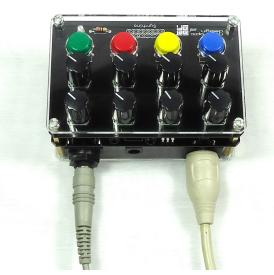
Synthino can be controlled externally with a MIDI keyboard, the device listens on all channels for MIDI notes and responds accordingly to the pitch note on and note off. The Synthesizer portion controls the current playing channel. Standard 5 pin MIDI DIN cable must be used. Shown with Audio and MIDI cables connected.
