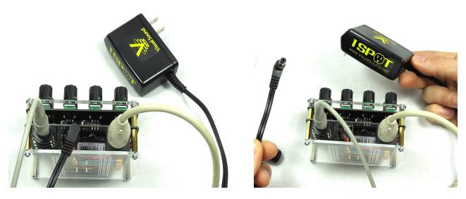
We recommend the use of a 1SPOT $^{\text{\tiny{M}}}$  guitar effects power adapter ( NOT INCLUDED ) or any other approved 9 volt adapter from the Synthino.com website for powering the unit during prolonged periouds of time. Power supply must be at least 500 mA Tip -.
